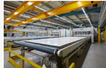
'SMART' GRP sidewall during the production process.
